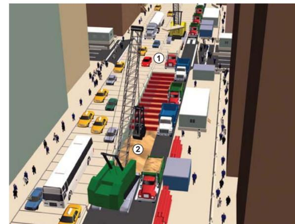
Most of New York City's subway system was built using the cut-and-cover technique. With this method, a trench is cut in the street, the soil is supported by
