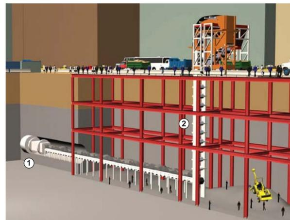
Much of the Second Avenue Subway will be built using tunnel boring technology, in which a powerful circular cutting machine drills a tunnel in rock or soil with minimal disruption to the street (1). The excavated material is then taken to street level and removed by truck (2). Tunneling will be done through bedrock wherever possible, which is quicker and more cost effective than mining or cut-and-cover.
